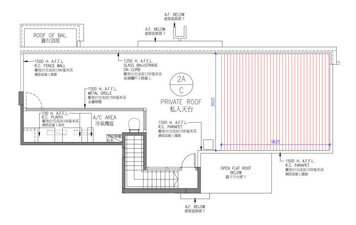
RECYCLE TIMBER DECK 100mm (H) 100mm(高)環保木甲板
