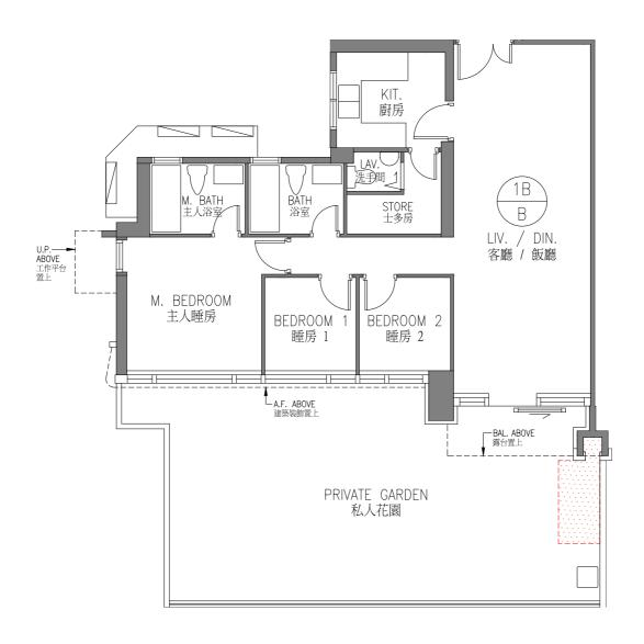
COMMON AREA FOR MAINTENANCE OF DRAIN PIPES (WITH 75mm (H) PLINTH WITH AN ADDITIONAL SIGNAGE INSTALLED PERMANENTLY WITH TEXT "MAINTENANCE AREA KEEP FREE AT ALL TIMES" TO DISTINGUISH PRIVATE GARDEN AND NOTIONAL COMMON AREA FOR MAINENANCE OF DRAIN PIPES) 供维修排水管的公共區域(75毫米高底座,並附有永久固定的標示牌,上面寫有『保持维修區域暢通』字樣以區分私家花園及維修排水管的公共區域。)
