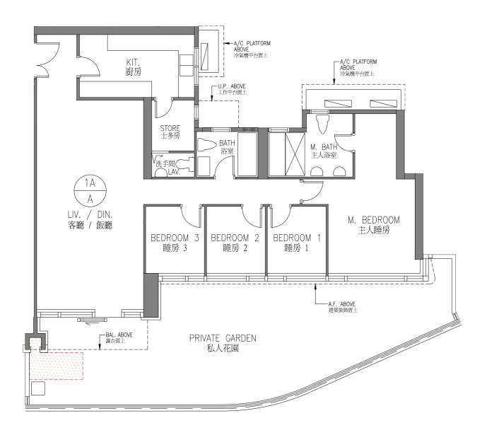
COMMON AREA FOR MAINTENANCE OF DRAIN PIPES (WITH 75mm (H) PUNTH WITH AN ADDITIONAL SIGNAGE INSTALLED PERMANENTLY WITH TEXT "MAINTENANCE AREA KEEP FREE AT ALL TIMES" TO DISTINGUISH PRIVATE GARDEN AND NOTIONAL COMMON AREA FOR MAINENANCE OF DRAIN PIPES) 供維修排水管的公共區域(75毫米高底座,並附有永久固定的標示牌,上面寫有『保持維修區域轉通』字模以區分私家花園及維修排水管的公共區域。)
