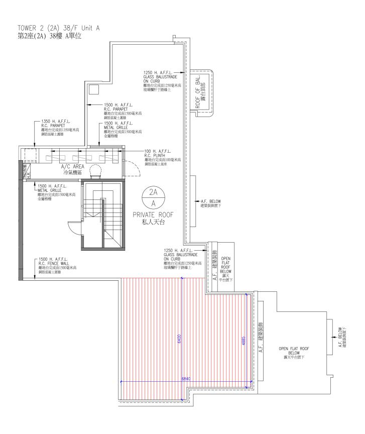
RECYCLE TIMBER DECK 100mm (H) 100mm(高)環保木甲板
