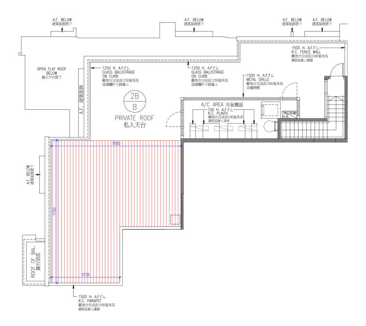
RECYCLE TIMBER DECK 100mm (H) 100mm(高)環保木甲板
